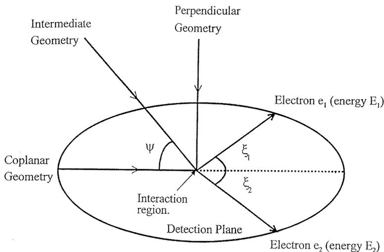
**Figure 1.** The (e, 2e) coincidence geometry used in the present experiments, showing the coplanar, intermediate and perpendicular plane geometries. The gun angle  $\psi$  is the angle between the detection plane and the direction of the incident electron beam. The symmetric scattering angles  $\xi$  in the detection plane are also shown. In the present studies  $E_1 = E_2$ ,  $\xi_1 = \xi_2$ .
