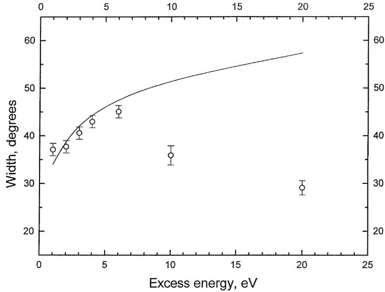
**Figure 3.** The dependence on excess energy of the width of the central peak in the  $(e, 2e)$  differential cross section in the perpendicular plane. The data points are obtained from the present results and those of Hawley-Jones *et al* (1992) and Murray *et al* (1992b), while the curve is derived from the 'extrapolated' Wannier model discussed in the text.
