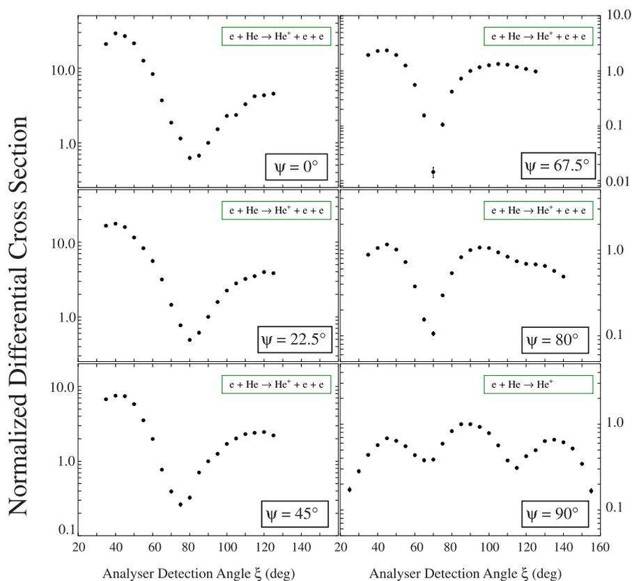
**Figure 4.** Ionization differential cross sections for helium at 64.6 eV incident energy shown on a logarithmic scale. The incident electron beam angle was varied over six selected angles from coplanar geometry ( $\psi = 0^\circ$ ) to the perpendicular plane geometry ( $\psi = 90^\circ$ ). The results are normalized to unity at the common point  $\xi = 90^\circ$ .
