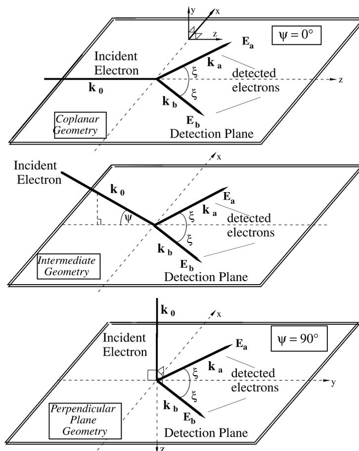
**Figure 1.** The experimental geometry, showing the evolution from coplanar to perpendicular plane geometry (a)–(c). The angle  $\psi$  is defined as the angle between the detection plane and the direction of the incident electron beam. The scattering angle  $\xi$  is defined as the symmetric electron scattering angle in the detection plane.
