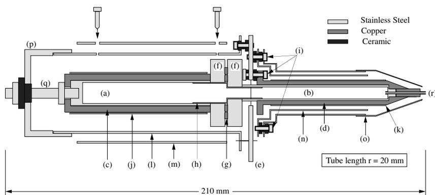
**Figure 1.** Scaled diagram of the oven: (a) body; (b) nozzle; (c) body heater; (d) nozzle heater; (e) oven holding and centring plate; (f) flanges; (g) copper gasket; (h) protective sleeve for copper gasket; (i) ceramic insulated stainless steel screws; (j, k) heating coils cover; (l) inner and (m) outer shield on body; (n) inner and (o) outer shield on nozzle; (p) end-cup locked onto the inner body shield; (q) Macor insulated M5 stud.
