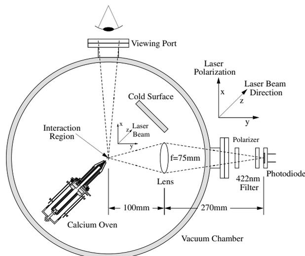
**Figure 3.** Schematic diagram of the experiment in the test chamber, showing the position of the oven, fluorescence collection optics and cold surface for deposition of the atomic beam.
