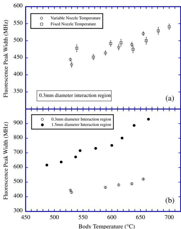
**Figure 6.** (a) Measured Doppler width as a function of body temperature. Open circles: both body and nozzle temperature are varied; open squares: nozzle is kept at a constant temperature of 710 °C. Fluorescence is detected from an interaction region of diameter 0.3 mm. (b) Both body and nozzle temperature are varied and fluorescence is detected from interaction regions of different size. Open circle: interaction volume of diameter 0.3 mm. Full circle: interaction volume of diameter 1.5 mm.
