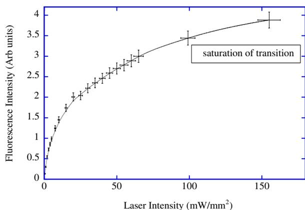
**Figure 8.** Variation of fluorescence intensity (and hence number density of excited atoms) as a function of the intensity of the laser radiation driving the transition.
