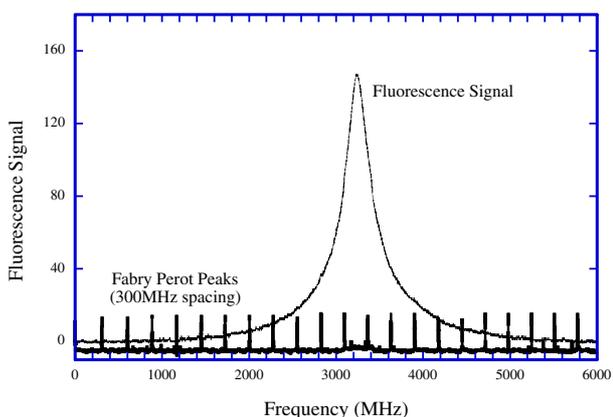
**Figure 5.** Doppler profile measured at a temperature of  $T = 530^\circ\text{C}$ . Fabry–Perot signals with peaks at a separation of 300 MHz used for calibration of the frequency scale are also shown for reference.
