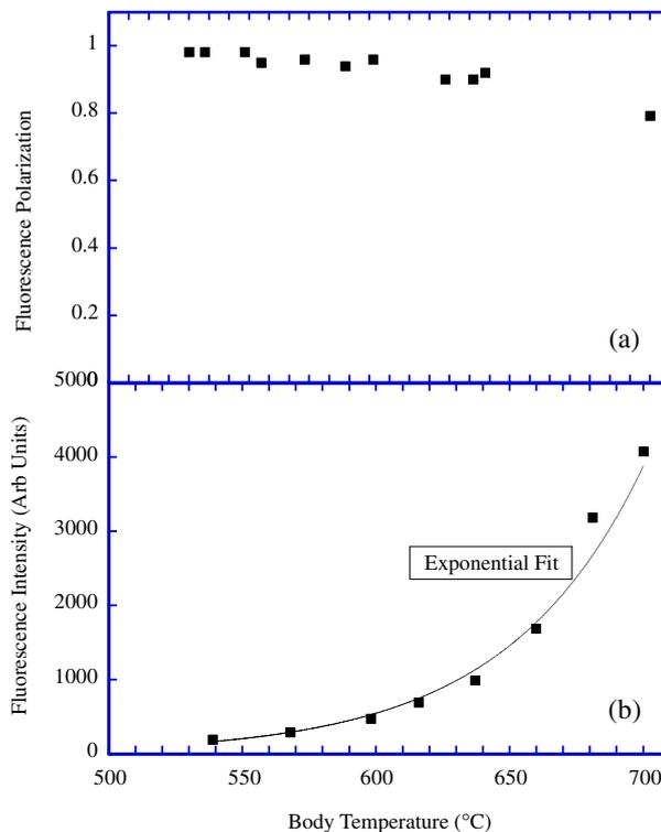
**Figure 7.** Polarization (a) and intensity (b) of the emitted fluorescence as a function of oven temperature. Significant depolarization occurs at temperatures in excess of 650 °C. The intensity and hence atomic beam density in the interaction region are seen to increase exponentially with temperature.
