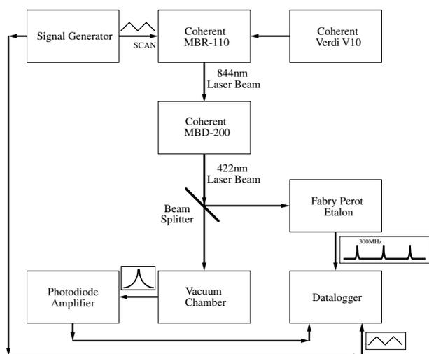
**Figure 4.** Block diagram showing the data collection electronics. The laser frequency is controlled by the signal generator and is monitored by the 300 MHz Fabry–Perot etalon. The fluorescence, etalon peaks and signal generator output are logged by a Pico Technologies datalogger.
