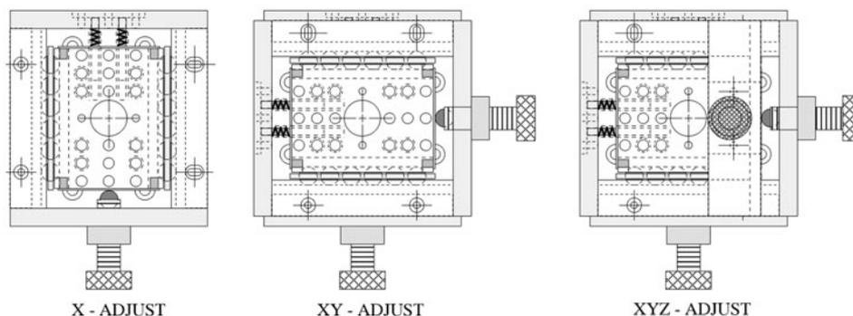
**Figure 2.** The translator configured as an  $x$ -,  $xy$ - and  $xyz$ -translator.
