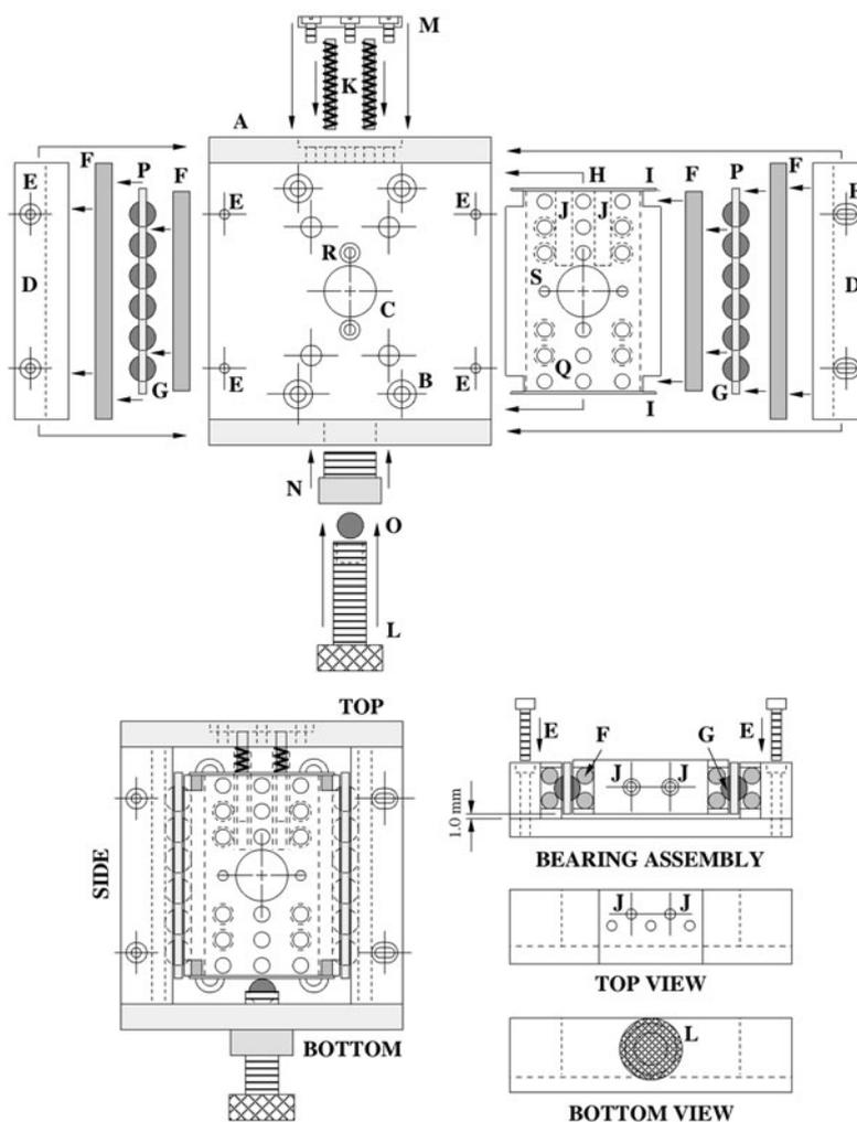
**Figure 1.** The translator detailing the individual components (A–S) as an exploded view, and showing the full assembly, bearing assembly and top and bottom view. For details, see text.
