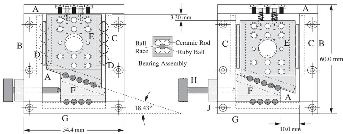
**Figure 2.** The new translator which uses a combined wedge drive assembly and linear bearing. The two extreme positions of the wedge and sliding table which drives in the  $\pm z$  direction are illustrated. The inset shows the bearing assembly constructed from four ground and polished ceramic rods together with highly polished ruby balls. For details, see the text.
