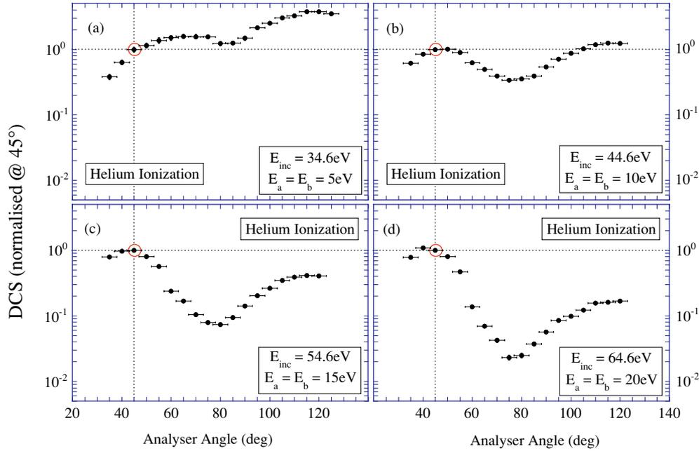
**Figure 5.** Comparative experimental results for ionization of He in a coplanar symmetric geometry for excess energies from (a) 10 eV to (d) 40 eV. The results are again normalized at  $\theta = 45^\circ$ .
