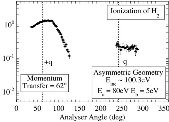
**Figure 6.** Experimental results for ionization of  $H_2$  in a coplanar asymmetric geometry for an electron of energy 80 eV forward scattered at an angle  $\theta_a = 35^\circ$ . The low energy electron of energy 5 eV is detected as a function of the angle  $\theta_b$ . The angle of the momentum transfer vector  $\mathbf{q} = \mathbf{k}_i - \mathbf{k}_a$  is also shown.
