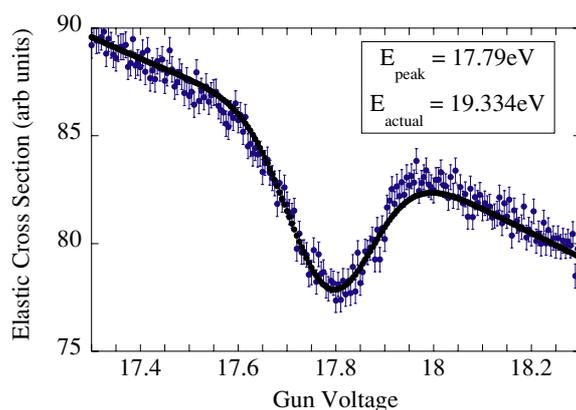
**Figure 2.** The elastic resonance in helium at 19.334 eV, measured at a scattering angle of 45°. The measured energy of the resonance is 17.79 eV, indicating that an offset of 1.54 V is present in the electron gun.
