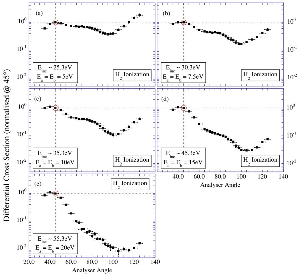
**Figure 4.** Experimental results for ionization of  $\text{H}_2$  in a coplanar symmetric geometry for excess energies from (a) 10 eV to (e) 40 eV. The results are normalized at  $\theta = 45^\circ$ . Horizontal error bars indicate the angular acceptance of the spectrometer. For details, see text.
