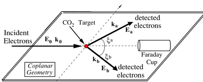
**Figure 1.** The (e, 2e) spectrometer configured in a coplanar geometry. The experiment is carried out in a symmetric geometry, where  $\xi_a = \xi_b = \xi$  and  $E_a = E_b$ .
