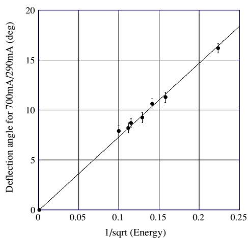
**Figure 4.** Calibration curve showing the deflection angle as a function of incident energy at a current of 700 mA/−290 mA in the MAC coils. A linear fit has been made to the data. For details, see the text.
