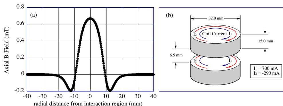
**Figure 2.** (a) The predicted axial magnetic field from the MAC device, showing the field in the interaction region and at a radial distance from the centre, for a coil current of 700 mA/−290 mA. The field is seen to be zero at  $r = 35$  mm, which is the distance to the entrance of the analyser lenses. (b) Representation of the coils, showing the direction of the currents for the inner and outer coils, together with the actual size of the MAC device.
