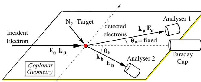
**Figure 1.** The coplanar asymmetric geometry, where one of the analyser angles is fixed in space.
