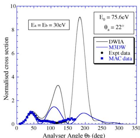
Fig. 5. Comparison of theory and experiment for coplanar asymmetric ionization studies from  $N_2$ . The experimental data was collected both with and without the MAC device operating. The calculation shows the results for a distorted wave impulse approximation (DWIA) and a molecular three-body distorted wave approximation (M3DW). Agreement between theory and experiment is poor, except for forward scattering.
