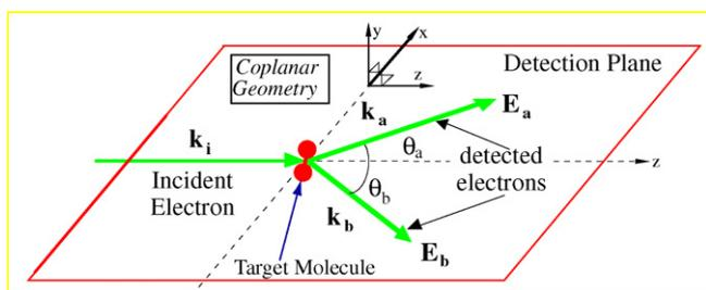
Fig. 1. Coplanar symmetric geometry, showing the direction of the scattered and ejected electrons following the collision.
