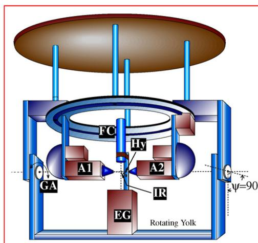
Fig. 2. The (e,2e) spectrometer in Manchester. The electron gun (EG) is shown in the perpendicular plane ( $\psi = 90^\circ$ ), and can rotate around the gun axis (GA) to a coplanar geometry ( $\psi = 0^\circ$ ). Analysers A1, A2 rotate in the horizontal detection plane with an axis through the interaction region (IR). The gas effuses from a hypodermic needle (Hy), the electron beam being dumped into a Faraday cup (FC).
