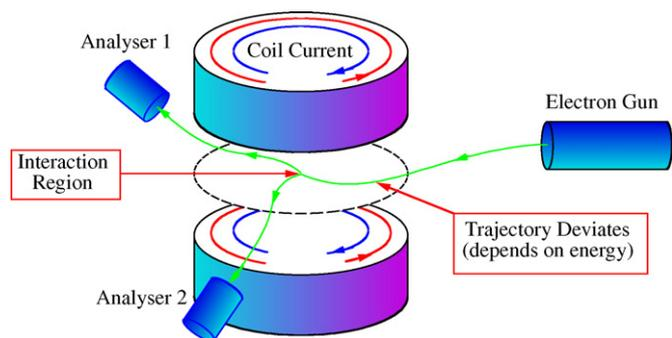
Fig. 3. The MAC device installed into the spectrometer. The coils are wound such that the magnetic field at the gun and analysers is zero. The field deviates incident and outgoing electrons according to their velocity, and so allows the angular range of the spectrometer to be extended.
