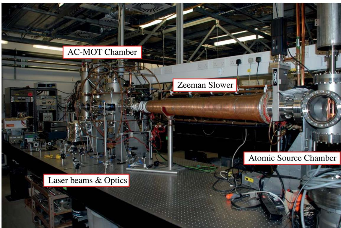
One of the two atom cooling and trapping instruments in Manchester, showing the source chamber (right), Zeeman slower (centre) and trapping chamber (left) where collision and ionization experiments are carried out.
