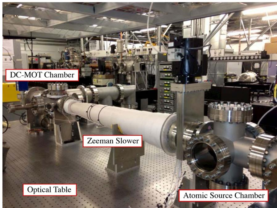
The new cooling and trapping source being built in Manchester to produce an ultra-cold electron beam for injection into new types of accelerators, Free Electron Lasers and for materials characterisation using electron diffraction. The source will produce an electron beam with an energy resolution several orders of magnitude better than conventional sources.
