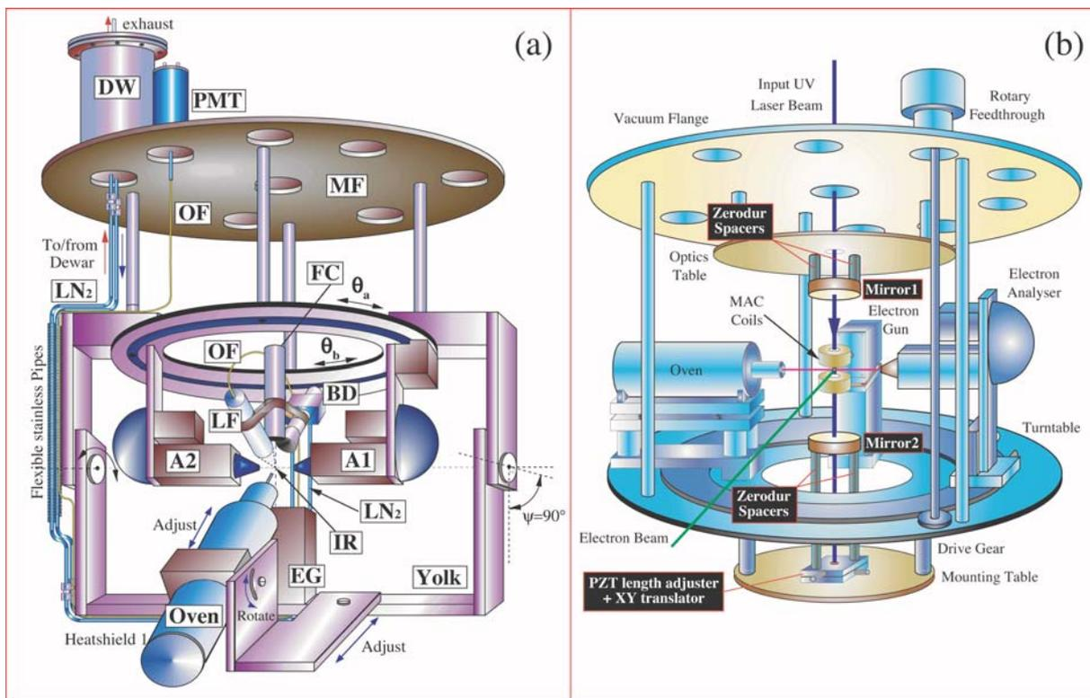
Two of the electron spectrometers for ionization and excitation studies of laser-prepared targets developed in Manchester. In (a), two detectors (A1,2) are used to detect electrons arising from the interaction (an e,2e process). In (b), a Magnetic Angle Changing (MAC) device controls the direction of incident and super-elastically scattered electrons from laser prepared targets, excited in a resonance enhancement cavity (Mirrors 1 & 2).
